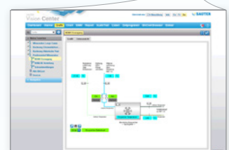
Visualisation of the heating and cooling systems in Winnenden with use of ice storage and waste heat and solar absorbers for ice storage regeneration.
