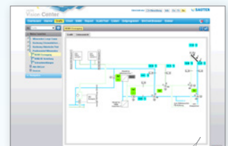
Visualisation of controls for the wood chip heating system in Paulinenhof with possible backup support from an oil boiler.
