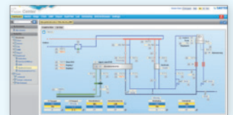
Regulation and monitoring of the cooling system in the Bethesda Hospital in Hoogeveen
