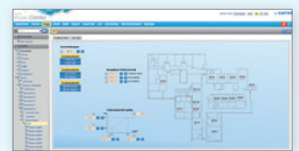
Temperature monitoring and regulation of the rooms in the Scheper Hospital in Emmen
