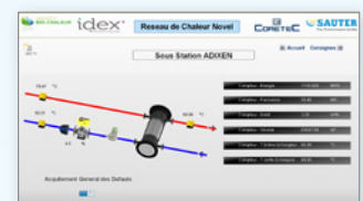
Visualisation of a substation with all the main meter values (e.g. energy, pressure, water volume, temperature).
